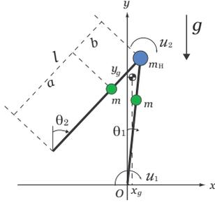
Fig. 1. Model of the compass gait biped
